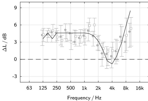
**Figure 4:** Auditory-canal level difference between binaural listening to diotic headphone and frontal loudspeaker presentation of pure tones at equal loudness (3.5 m distance to the loudspeaker, 70 dB SPL at the listening position, free sound field). Solid black contour: Predictions of the working model proposed here, implemented based on DIN 45 631 (1991). Light gray: Quartiles from Fastl et al. (1985): filled circles indicate “closed”, white squares “open” headphones.
