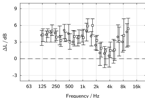
**Figure 1:** Auditory-canal level difference between binaural listening to diotic headphone and frontal loudspeaker presentation of pure tones at equal loudness (3.5 m distance to the loudspeaker, 70 dB SPL at the listening position, free sound field). Quartiles from Fastl et al. (1985): filled circles indicate “closed”, white squares “open” headphones.
